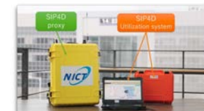
Figure 5-10: Configuration example of portable SIP4D and operating terminal
